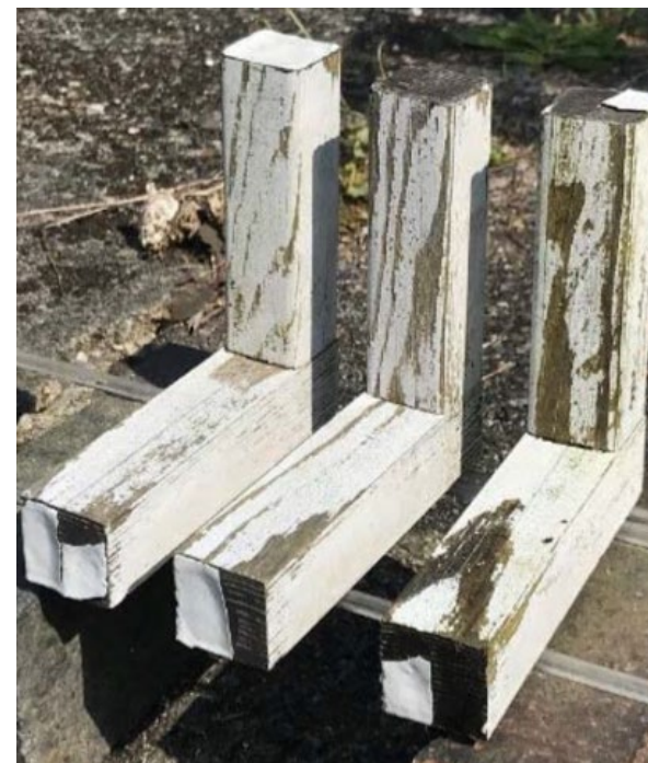
The acetylated L-joints after 20 years of exposure
