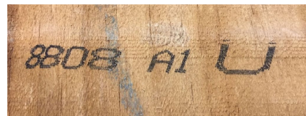
The U mark indicates that Accoya is certified under the German certification system for solid wood in structural applications
