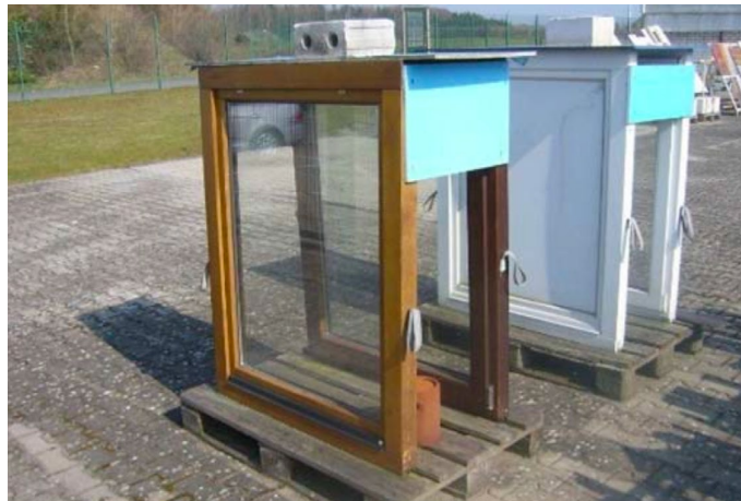
The test rigs after 10 years of exposure
